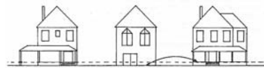
New construction must maintain foundation heights with adjacent structures. The foundation of the house in the center is too low.
